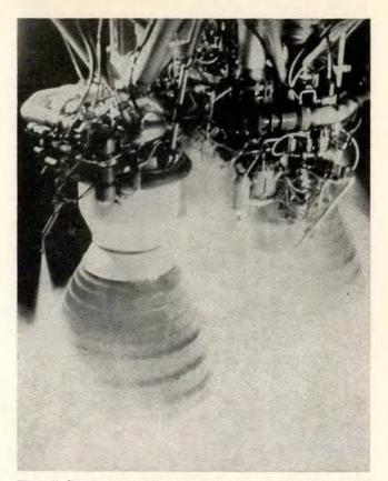
Titan II first stage engine test firing. During SLAP approximately every third engine was static fired prior to teardown to test performance.
